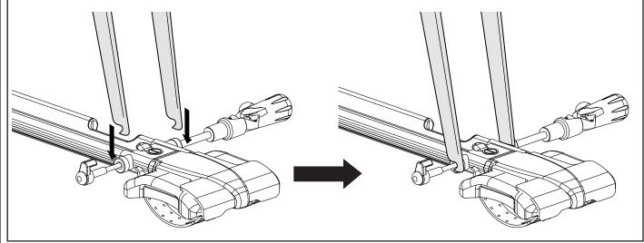
Twist handle clockwise to tighten the quick release skewer. Close the handle by flipping it 90 degrees to the closed position. If it is too loose, open the handle and turn it like a screwdriver (clockwise to tighten, counter clockwise to loosen), and close the handle again. Re-adjust until a firm and positive snap is felt when closed. If locks have been purchased or provided, the cover can now be locked.
