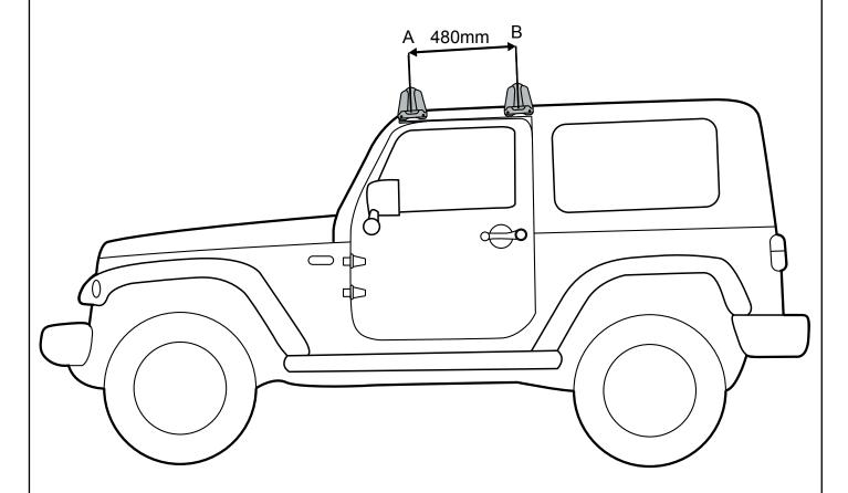
Measure forward 100mm (3,15/16") from the end of the rain gutter to the centre of the rear leg then a further 480mm (18,29/32") forward to the centre of the front leg, see diagram below. Progressively tighten each of the M6 screws. Tighten to 3-4 Nm (2-3 lbs/ft). Do not over tighten.
