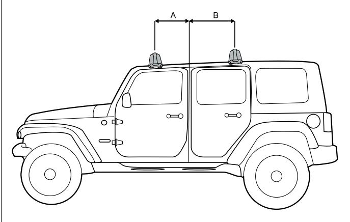
Measure forward 300mm (11,13/16") from centre of door jambs to centre of front leg. Measure rearward 500mm (19,11/16") from centre of door jambs to centre of rear leg, see diagram below. Progressively tighten each of the M6 screws. Tighten to 3-4 Nm (2-3 lbs/ft). Do not over tighten.
