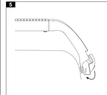
Swing the support leg strap under the gutter. Make sure that the strap is fully located under the gutter.
