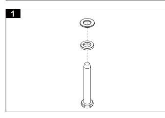
Assemble spring washer and flat washer onto M6 x 40mm security screws.
