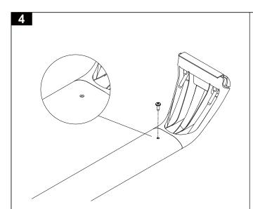
From underside of the crossbar fasten the 10G self tapping screw through the crossbar and into the leg. Repeat this process for all legs.
