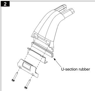
Insert security screw assembly through the cover strap, and fasten to the dowel nuts which are located in the support leg. Turn the screw so that it just engages into the dowel nut.
