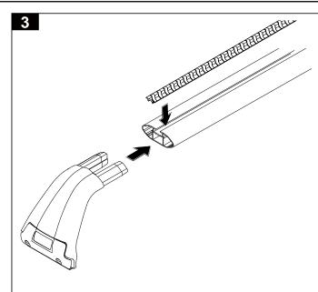
Locate support legs into the crossbar, a rubber mallet can be used to knock the legs in.
