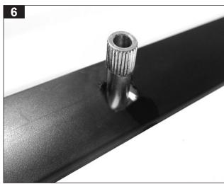
Re-install left & right roof ditch mould. Fasten all four studs.
