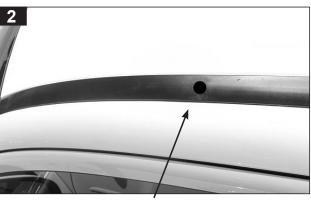
Front left hole position shown. Remove roof ditch mould.
