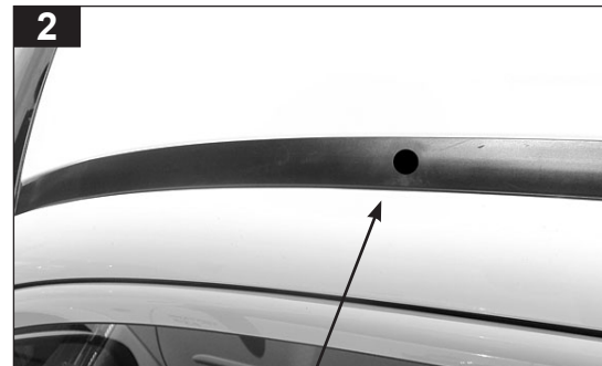
Front left hole position shown. Remove roof ditch mould.
