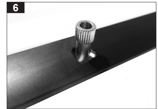
Re-install left & right roof ditch mould. Fasten all four studs.
