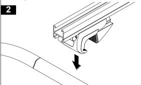
Pull the inner and outer clamp legs together around the rails. Adjust the heavy duty crossbar so that the crossbar over hang is equal both sides, finger tighten the crossbar attachment bolt.
