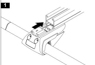
Using the security allen key provided, tighten both leg clamp bolts equally, the outer clamp leg will move in towards the inner clamp leg. The leg assembly on some vehicles will lift as the security bolts are tightened. Fully tighten the security bolts. Check that the outer clamp leg rubber seal has folded out over the roof rails.
