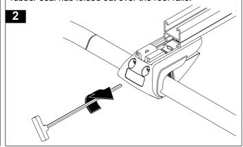
Check the crossbar over hang (A) (B) is equal on both sides, re-adjust if required. Fully tighten the security leg clamp bolts, and then the crossbar attachment bolts using a 13mm spanner. **Do not over tighten.**
