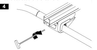
Check the crossbar over hang (A) (B) is equal on both sides, re-adjust if required. Fully tighten the security leg clamp bolts, and then the crossbar attachment bolts using a 13mm spanner. **Do not over tighten.**
