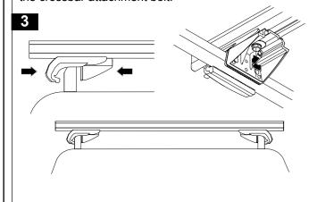
Using the security allen key provided, tighten both leg clamp bolts equally, the outer clamp leg will move in towards the inner clamp leg. The leg assembly on some vehicles will lift as the security bolts are tightened. **Do not fully tighten the security bolts** as final tightening occurs later. Check that the outer clamp leg rubber seal has folded out over the roof rails.
