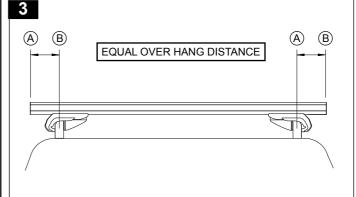
Using a rubber mallet knock the end caps into the crossbars, insert the rubber buffer strip fully into the crossbar as per the diagrams. Check the buffer strip is fully inserted.
