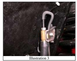
23. Install track bar into factory mount using OEM 30mm bolt. Torque to 135 ft./lbs
