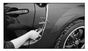
3.) Hold down the Quarter Molding in the center and pull the rear tab toward the bottom of the vehicle as shown below. Apply light pressure to the insert where the lining has been removed.
