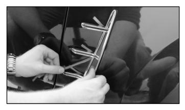
5.) Pull the remaining three tabs toward the front of the vehicle as shown below. Apply light pressure to the insert where the lining has been removed.
