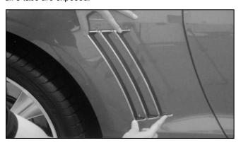
4.) Once quarter molding is properly aligned, press firmly on the quarter molding where the lining has been pulled back as shown below. This will hold the quarter molding in place while you pull the remaining tabs.
