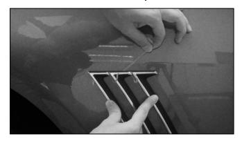
**6.)** Pull the three middle tabs toward the bottom of the vehicle starting with the rear most tab as shown below. Be sure quarter molding remains properly aligned when pulling tabs. Apply firm pressure where lining has been removed.
