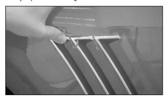
5.) Pull the entire top tab toward the front of the vehicle. Be sure that Quarter Molding remains properly aligned as you pull the tab. Apply firm pressure where lining has been removed. Caution: Use extreme care when pulling liner so as not to tear the liner. See Installation Tips.
