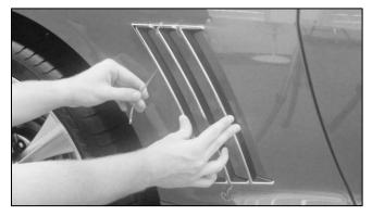
7.) Pull the bottom tab toward the front of the vehicle as shown below. Apply firm pressure where the lining has been removed.
