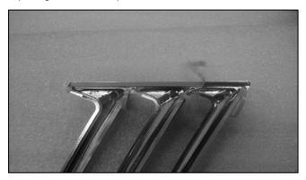
3.) Align quarter molding on the vehicle over the existing louvers impressions on the quarter panel as shown below. Quarter molding should be flush with vehicle quarter panel. Be sure all 5 tabs are exposed.
