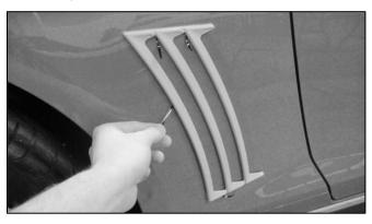
10.) Remove the bottom lining by pulling the bottom tab toward the front of the vehicle as shown below. Apply firm pressure where the lining has been removed.
