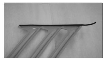
**3.)** Apply a piece of tape to the bottom edge surface on the inside of the quarter molding as shown below. Leave a 1" tab at the rear of the quarter molding.
