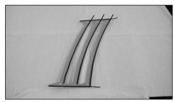
**5.)** Use a razor blade to cut the extra tape from the five 1" tabs leaving just the liner. These tabs will aid in removing the liner during installation.
