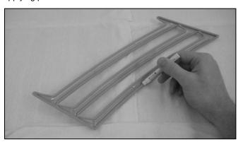
2.) Using the included tape, apply a piece of tape to the top edge surface on the inside of the quarter molding as shown below. Leave a 1" tab at the rear of the quarter molding. Caution: Use caution when applying tape to the quarter moldings. Tape will not be able to be removed after applying to quarter molding surface.
