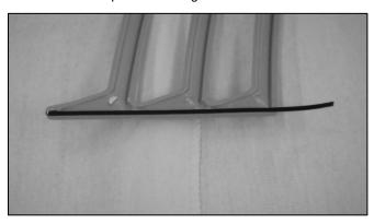
4.) Apply a piece of tape to the rear edge surface on each of the three gills as shown below. Leave a 1" tab at the top of the quarter molding.
