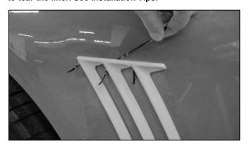
9.) Remove the three middle linings by pulling the three middle tabs toward the bottom of the vehicle starting with the rear most tab as shown below. Be sure quarter molding remains properly aligned when pulling tabs. Apply firm pressure where lining has been removed.
