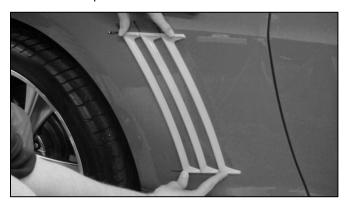
8.) Once quarter molding is properly aligned, remove the top lining by pulling the top tab toward the front of the vehicle as shown below. Be sure that Quarter Molding remains properly aligned as you pull the tab. Apply firm pressure where lining has been removed.
