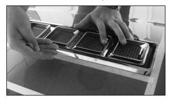
**6.)** Pull the outside tab toward the front of the vehicle as shown below. Apply firm pressure where the lining has been removed.
