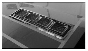
**4.)** Once the vent is properly aligned press down firmly on the vent where the lining has been removed as shown below. Apply the pressure to the painted black surface. This is the surface directly above the tape.
