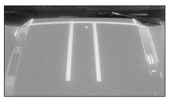
**2.)** Once the hood is masked off, remove the tape lining from the rear of the vents as shown below. The rear of the vents is the end without the drain holes.
