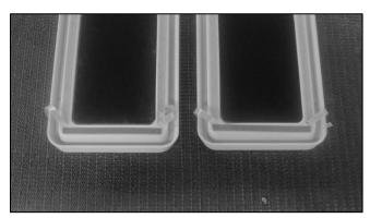
3.) Align one of the vents on the vehicle hood using the masking tape that you laid out on the hood as shown below. Be sure all three remaining tabs are exposed.
