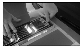
5.) Pull the inside tab toward the front of the vehicle as shown below. Be sure vent remains properly aligned as you pull the tab. Apply firm pressure where the lining has been removed. Again, apply the pressure to the painted surface.
