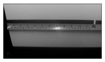
**8.)** Align quarter scoop on the quarter panel so that the bottom edge of the quarter scoop is parallel with the top edge of tape from step 7. Front edge of quarter scoop should be aligned with line made in step 8. See picture below.
