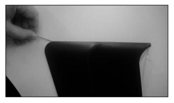
**10.)** Now gently remove the front edge tape lining by pulling the tab towards the bottom of the vehicle as shown below. Apply light pressure where the tape has been exposed.
