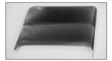
3.) Apply a continuous piece of tape to the front edge of the flat perimeter surface on the inside of the quarter scoop as shown below. Leave 1" tab at the top front corner of the scoop as shown below. Entire perimeter of the quarter scoop should now be covered with tape.
