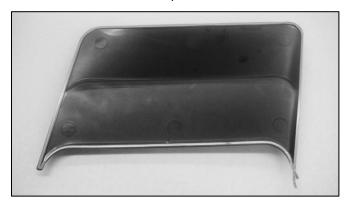
4.) Use a razor blade to cut the extra tape from the two 1" tabs leaving just the liner. These tabs will aid in removing the liner during installation.
