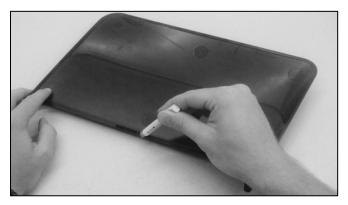
2.) Using the included tape, apply a continuous piece of tape to the bottom, rear, and top edges of the flat perimeter surface on the inside of the quarter scoop as shown below. Leave a 1" tab at the top front corner of the scoop as shown below. Caution: Use caution when applying tape to quarter scoops. Tape will not be able to be removed after
