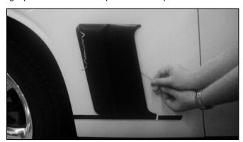
11.) Last, remove the rest of the outer lining by gently pulling the outer lining tab towards the bottom of the vehicle as shown below. Apply light pressure where the tape has been exposed.
