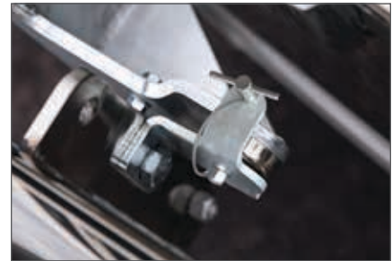
206492 safety pin adds security to the magnetic system
