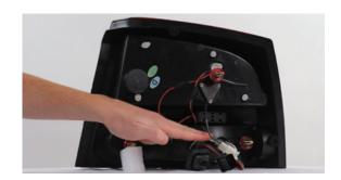
2. Disconnect your battery's negative battery terminal. Please note that some automobiles (such as newer GMs) have highly sensitive electrical systems. If such is the case, a failure to disconnect the battery before beginning installation may cause blown tail lamp fuses or other similar damages.
