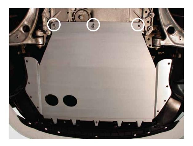
This skid plate is a direct replacement to the factory plastic engine cover. Remove the factory unit and install the aluminum skid plate using the factory hardware for the front and both sides. Use the (3) bolts and washers supplied with this kit to attach the back edge of the plate as shown in the photo above.
