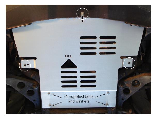
Remove the factory plastic splash guard and install the aluminum unit using the (3) factory screws circled and the (4) supplied bolts and washers.
