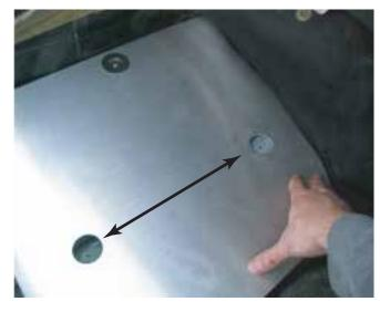
Install Track Mat into car and drill 3/8" holes into frame rail in the center of the Track Mat mounting holes.
