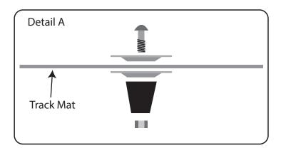
Attach rubber bumper to the mounting hole closest to the center tunnel of the car using the supplied M6 machine screw and (2)embossed washers. Note: The Track Mat goes between the 2 washers, both have the ebossed area facing down.
