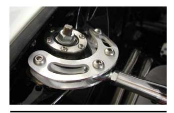
Install as shown above. Note: Drivers side top bracket is marked with a red dot on the top side Keep all bolts finger tight until installation is complete.
