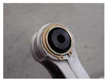
Step 4 - Install the C-clip making sure it is fully seated into the machined groove of the monoball cartridge. Reinstall the control arm into the car and repeat 3 more times. Enjoy your new Rennline product.
