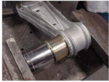
Step 3 - With a press or vise, press the monoball cartridge into the control arm opening using a large socket (or equivalent). Make sure that the cartridge is straight before applying pressure. DO NOT PRESS ON THE BLACK BUSHINGS.
