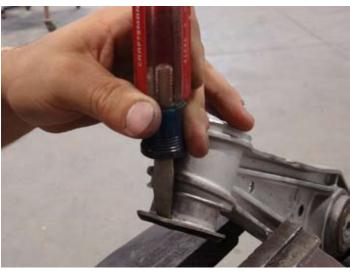
Step 1 - Once the control arms are out of the car, remove the factory aluminum cased bushings by using a chisel (or equivalent) and pound them out each side of the control arm as shown in photo. These bushings are a 2 piece design.
