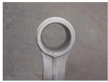
Step 2 - After the factory bushings have been removed, clean the control arm making sure it is free of any defects that may hinder the installation of the monoball cartridge sliding into the control arm opening.
