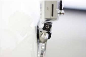
To install, Simply remove the tow loop from your Rennline Tow hook. Slide the GoPro mount onto the screw as shown in Photo 1 and tighten the supplied set screws using the supplied hex key. Next, reinstall the tow loop using the instructions included in the tow hook kit. Lastly mount the GoPro to the Rennline GoPro mount making sure to tighten the GoPro thumb screw tight enough.
