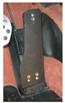
Place lifter plate onto factory pedal making sure that it is in the desired position. Adjust the reamed holes as required to position lifter plate. Drill the required mounting holes for your model using a 1/16" bit and attach using the supplied self tapping screws.
