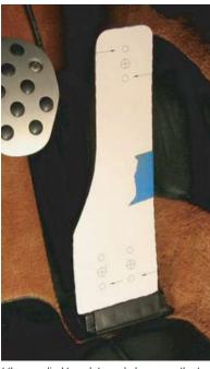
Cut out the supplied template and place over the top of the factory pedal in the desired position and attach with tape.
