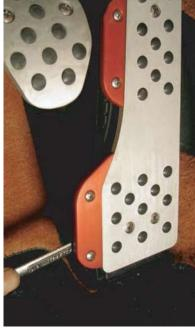
Lock pedal cover into desired position by tightening the (3) nuts on the back of the pedal cover using a 3/8" wrench.
