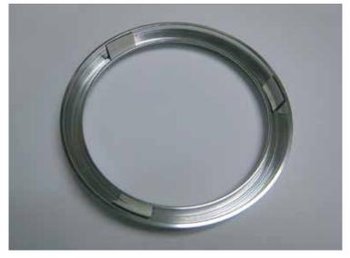
Cut the supplied tape into approximately 1/2" X 1/4" rectangles. Apply tape to the inside of each bezel as shown above.
