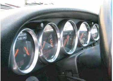
Thoroughly clean factory bezels removing any contaminates such as Armor All that may inhibit the tape to properly adhere to the surface. Remove the backing from the applied tape and install the aluminum bezels over the top of the factory bezels. To insure proper adhesion of the tape, apply equal pressure to all sides of the bezels. Note: This is an acrylic based tape, full adhesion will not be achieved for a few days after installation.
