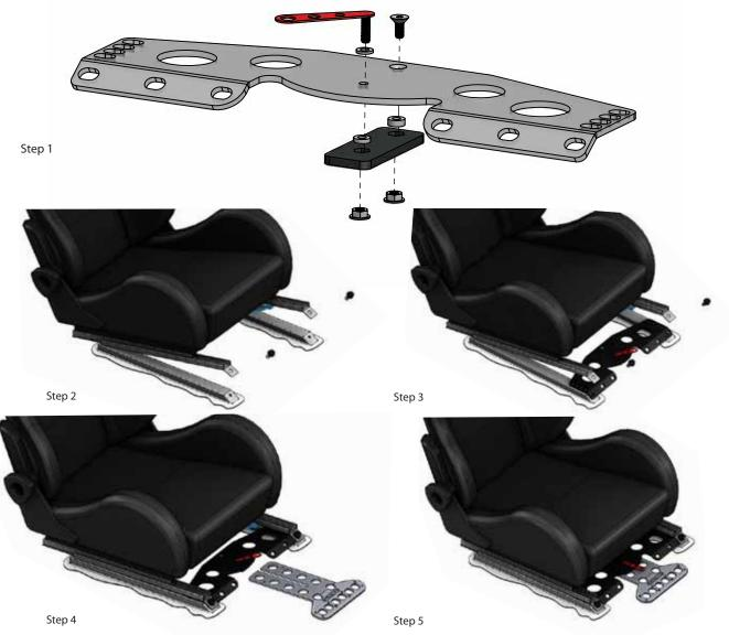
This mount may or may not work on both Drivers and Passenger seats depending on your model and options. Evaluate the clearance of the components under the seats to determine what seat you will be installing on. Some models will have wiring harnesses that may need to be moved and or secured to allow for adequate clearance.
