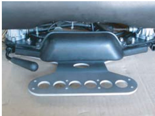
Step 8 - Reinstall plastic motor cover.
