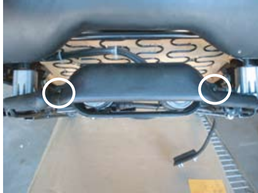
Step 2 - Remove plastic motor cover. Step 3-5 describes the installation of a stiffener plate that is designed for use in high vibration environments. Its not required but recommended. If your not using the stiffener plate skip to step 6
