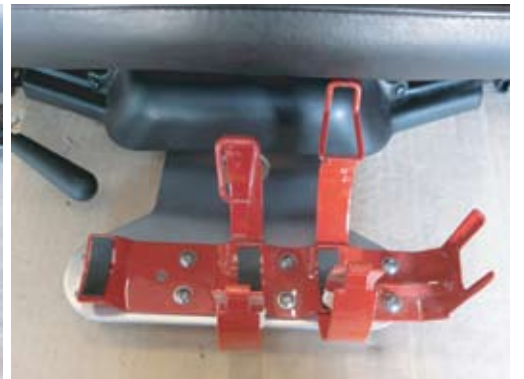
Step 9 - Install fire extinguisher bracket using the supplied (6) button head screws, washers and nuts. This mount was designed for a standard Hal Guard bracket. If your mounting holes are different you may need to drill your bracket to properly fit. Install seat into car.
