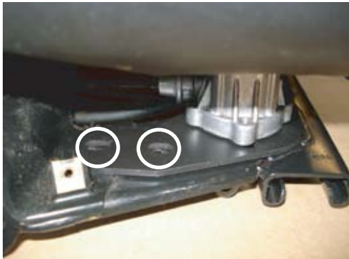
Step 4 - Insert stiffening plate between the actuator and the motor bracket. Install the supplied M6 X16mm bolts and washers as removed from step 3. Make sure that the (2) holes are aligned as shown above.
