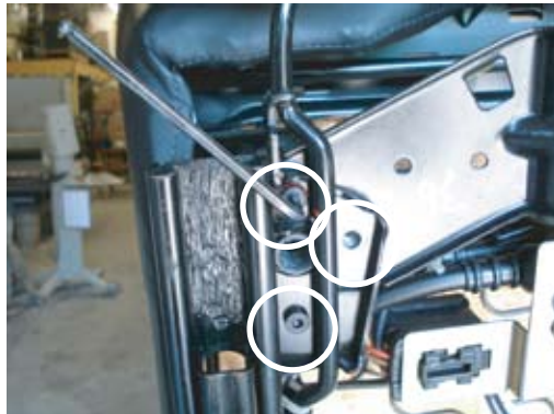
Step 5 - Repeat steps 3 & 4 on the other side of the seat. You must rotate the slider arm to access (2) of these mounting bolts.
