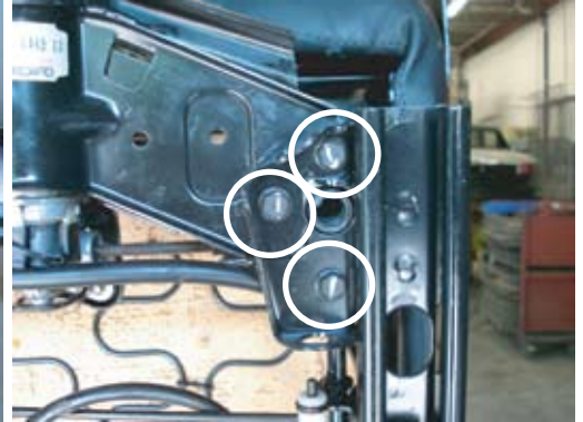
Step 3 - Remove the (3) M6 bolts that attach the seat actuator. Only remove one side of the seat at a time.
