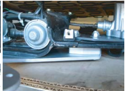
Step 6 - Install the fire extinguisher mount using the (2) aluminum spacers and the (4) 6mm X 35mm bolts, washers and nuts as shown. This mount can be flipped to adjust fire extinguisher height.
