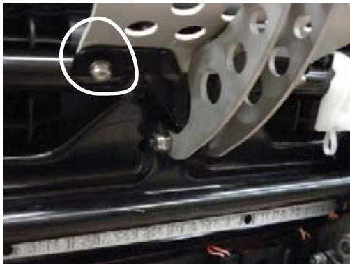
Step 3 - Attach the aluminum face plate to the seat and the S/S bracket as shown above using the supplied 8/32 button head screws, nuts and washers. Leave all hardware loose until everything is in place, and then tighten hardware.
