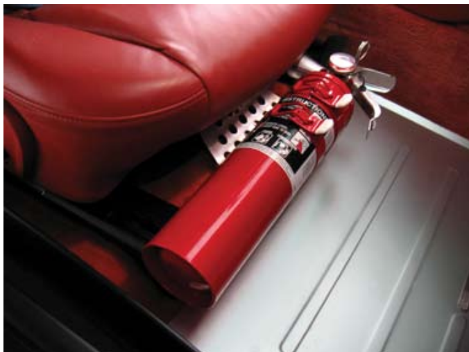
Step 3 - Attach the aluminum face plate to the seat and the S/S bracket as shown above using the supplied 8/32 button head screws, nuts and washers. Leave all hardware loose until everything is in place, and then tighten hardware.
