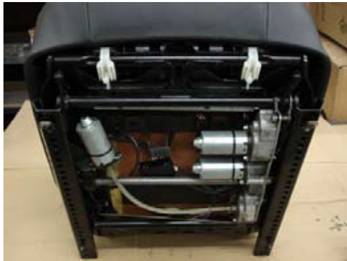
Step 1 - Remove seat from car and position it so you can access seat bottom as shown.
