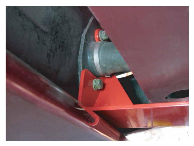
Mounts on top of factory bumper shock attachment point on all 1983-1991 944's using factory hardware.
