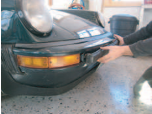
Step 1 - Remove front impact strip.
