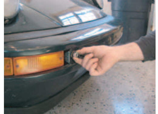
Step 3 - Remove (4) bumper bolts.
