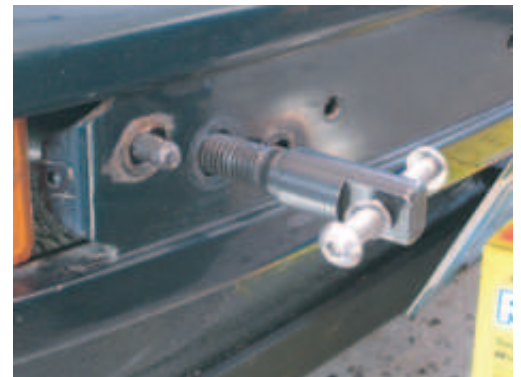
Step 9 - Place bumper onto car and check hole placement by inserting tow hook screw. Make adjustments as needed.
