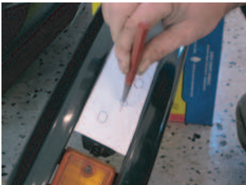
Step 7 - Using the supplied template. Align mounting holes and mark the toe hook screw hole location.
