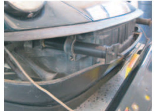
Step 6 - Install Rennline bumper shock. Note: On some early cars, the rear mounting hole is a smaller size than required. Ream hole to the appropriate size.
