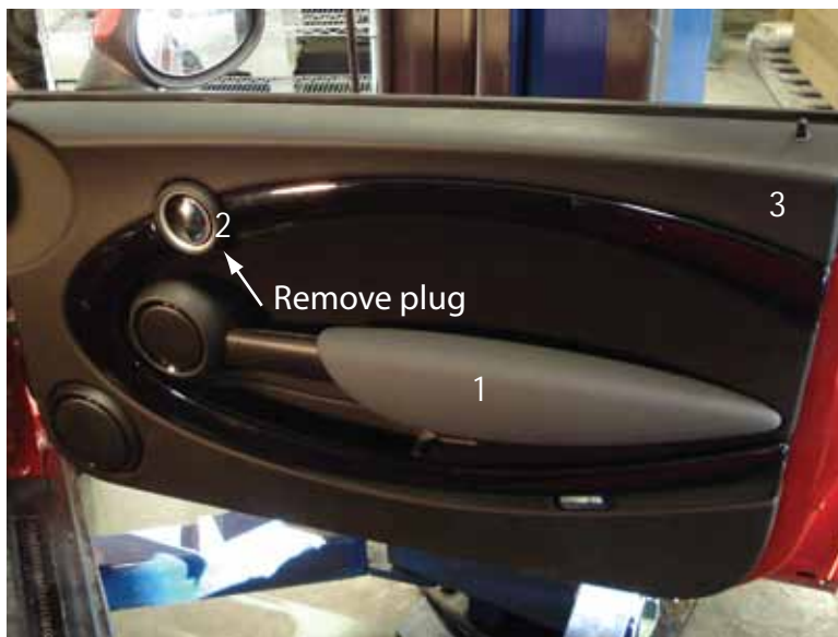
Step 1: Put window in the down position. Using a screw driver with tape wrapped around the tip, carefully pry off, (1) armrest, (2) handle surround (remove small plug at bottom) and the (3) main door card. See photo for locations. Don't be afraid, they do all just pull off.
