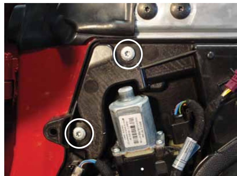
Step 4: Remove the (11) torx head screws located all the way around the door component housing. We have circled 2 of these for you in the photo above.
