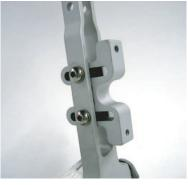
Step 2: Attach the (2) Lifter brackets as shown. We recommend installing them in the center as a starting position. Once the pedal is installed into car you can easily make the necessary adjustments. Note: for 924,944 and 968 cars see photo 3.
