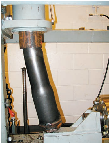
Competitor's 25K gooseneck fails longitudinal test at 11,500 lbs.
