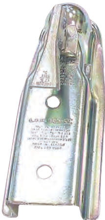
Fulton coupler after 336 hours salt spray testing.
