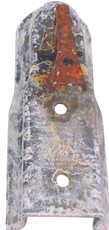
Competitor's coupler after 336 hours salt spray testing.
