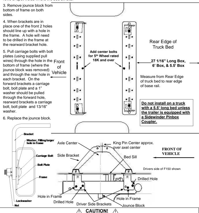
Check for obstructions before drilling. Failure to do so could result in damaged fuel or brake lines, structural members, etc. CEQUENT TOWING PRODUCTS does its best to communicate tow vehicle manufacturer changes; however, it is ultimately the responsibility of the installer to prevent damage due to installation.
