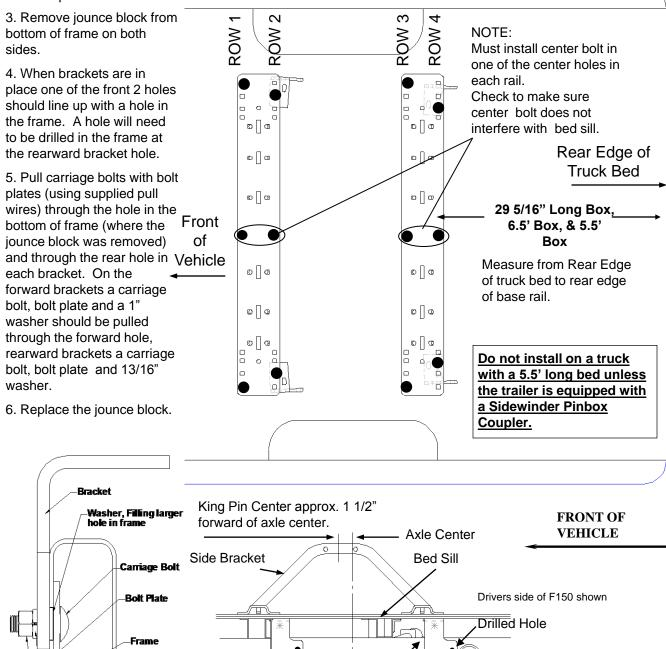
Drilled Hole Driver Side Brackets
