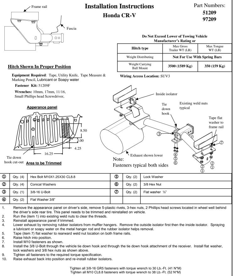
Note: check hitch frequently, making sure all fasteners and ball are properly tightened. If hitch is removed, plug all holes in trunk pan or other body panels to prevent entry of water and exhaust fumes. A hitch or ball which has been damaged should be removed and replaced. Observe safety precautions when working beneath a vehicle and wear eye protection. Do not cut access or attachment holes with a torch.
