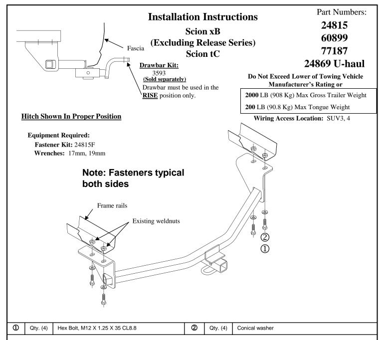
If present, remove the tie down brackets from vehicle frame rail. Return bolts and tie down bracket to owner.
