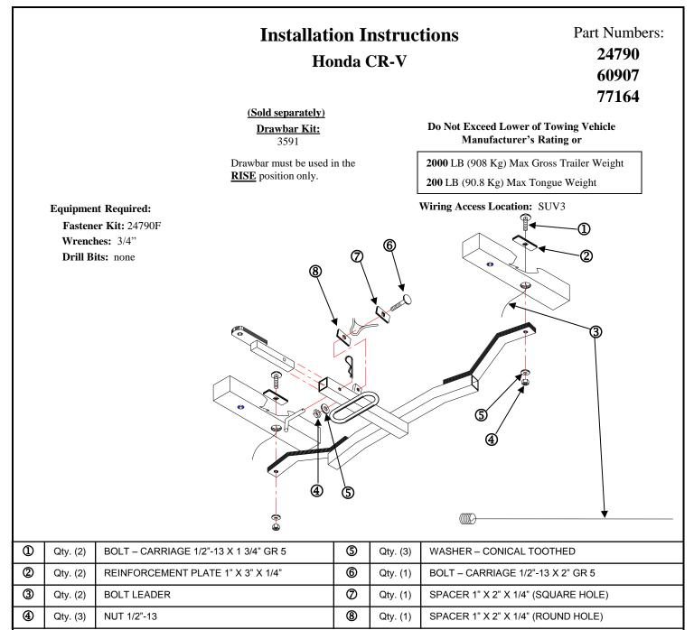
1. Thread bolt leader (3) onto 1 3/4" carriage bolt (1) and insert bolt leader through hole in reinforcing plate (2).
