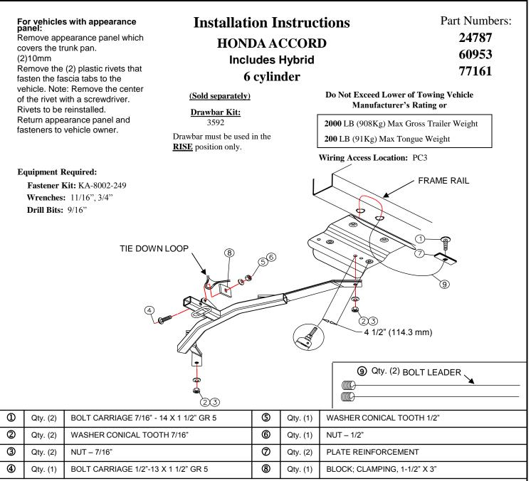
1. Lower exhaust by removing both rubber isolators from muffler hangers. Be careful not to allow mufflers to fall under their own weight. 2. Both heat shields will need to be marked and drilled 4 1/2" from the forward most hole on the frame channel. Mark holes then hold hitch in position to check. Refer to illustration for clarification. Remove heat shield to drill.
