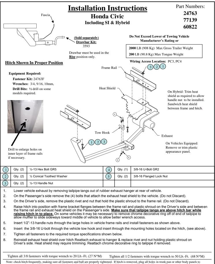
prevent entry of water and exhaust fumes. A hitch or ball which has been damaged should be removed and replaced. Observe safety precautions when working beneath a vehicle and wear eye protection. Do not cut access or attachment holes with a torch.
