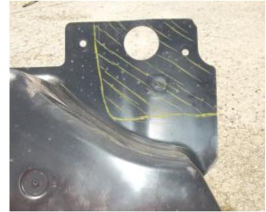
With the marker mark out the area to be trimmed, then using the Utility Knife trim the area.
