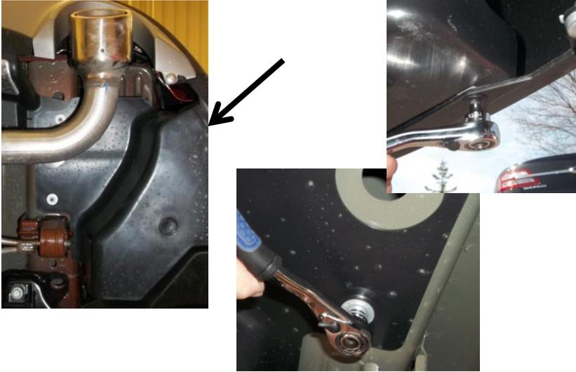
2. Lower the exhaust at the rubber isolators on both sides of the exhaust. Support the exhaust to prevent damage to the vehicle. Note: Spraying a lubricant or soapy water on the metal hanger rod and the rubber isolator helps removal.
