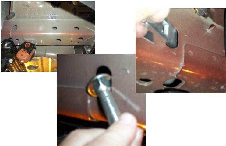
4. Pull the pull wire with fasteners into location through the hole. Leave pull wires attached. Repeat the same process on both frame rails. Push the fasteners back into the frame rails with the pull wire attached, to allow the hitch to go into position. See figure 2
