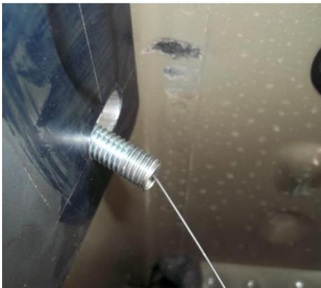
6. Feed conical washer over pull wire, using the washer to hold the bolt in place remove the pull wires and attach the hex nut. Tighten to hold hitch in place, repeat with all fasteners.
