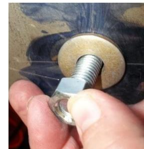
7. Hitch will tend to slant at a slight angle downward, push hitch straight up into frame and tighten hitch.
