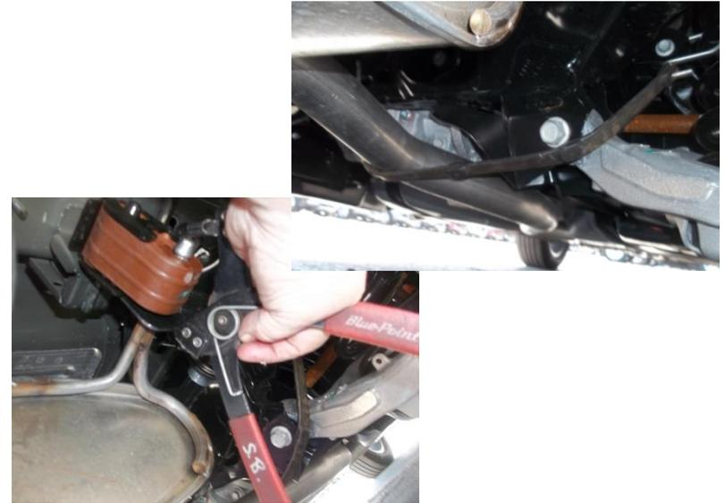
3. Feed the coiled end of the pull wire through rearward hole and out the access hole. Attach spacer and carriage bolt onto pull wire and feed the fasteners into location through the hole. Leave pull wires attached. Repeat the same process on the both frame rails. Note: it may be easier to install the carriage bolt head first. Repeat with the forward holes. Both frame rails. Note: carriage bolt tight fit into access hole may be necessary to use a file or wrench to open access hole. See figure 3.
