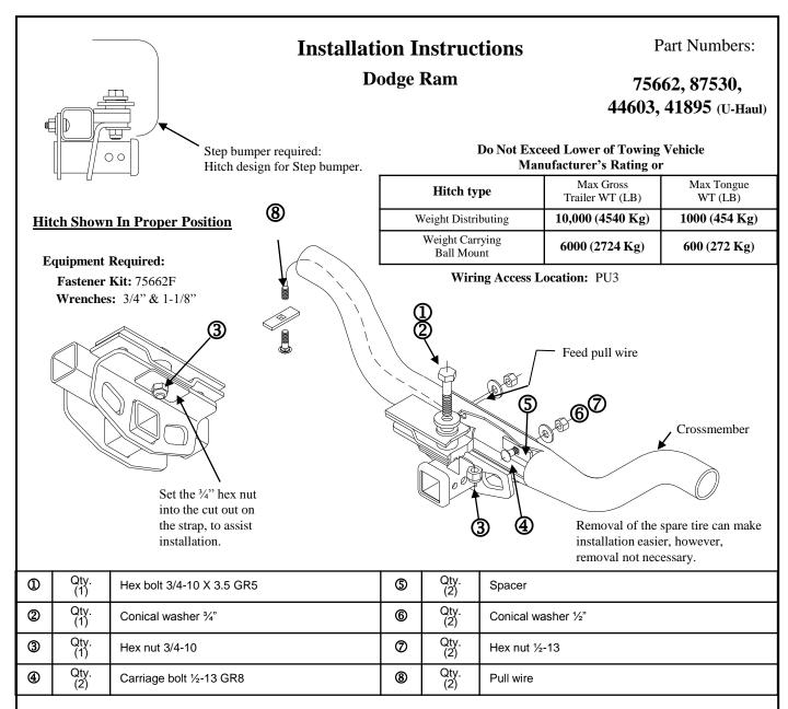
1. Removal of the spare tire can make installation easier, however, removal not necessary.
