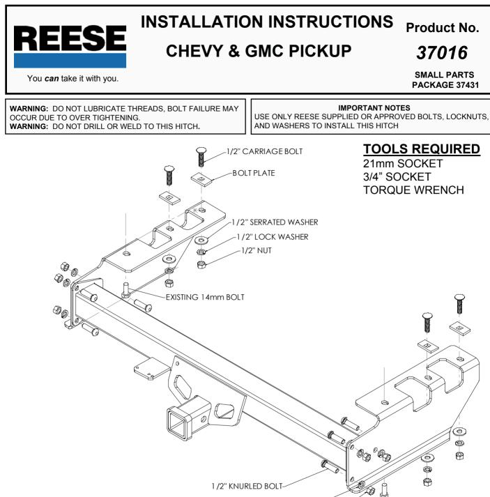
1. Remove the 14mm bolt from the bottom of the bumper bracket on both sides of the vehicle. Align the brackets with these holes and install the two existing 14mm bolts.
