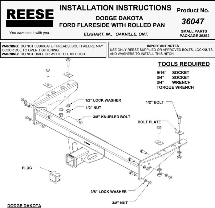
1. Assemble center section and side brackets (flanges out) with six 3/8" knurled bolts pointing outward. Install six 3/8" lock washers and six 3/8" nuts. Leave nuts slightly loose on bolt at this time.
