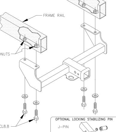
1. REMOVE TIE DOWN BRACKET AND BOLTS ON DRIVER'S SIDE AND RETURN TO VEHICLE OWNER.
