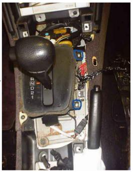
**2.** Unplug overdrive plug. It may be tucked under the shifter a little and held in place with some clips that just fold over.
