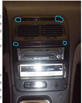
**5.** Pull out the ashtray and remove the bolt underneath it.
