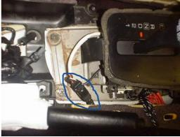
**3.** Remove the 2 screws on the front side of the shifter.
