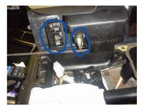
(passenger side of trim). Open the utility tray, and use a flat-blade screwdriver to pull up the front (largest) felt covering to expose three bolts. Remove these bolts.
