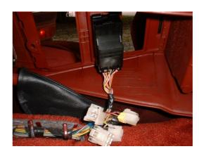
**5.** Remove the shift boot trim piece from the body of the console by pushing on the plastic clips that hold it in place. Pry off the clips holding shift boot (be careful, they like to fly), and remove the four screws holding the metal clamps in place. Remove the old boot.
