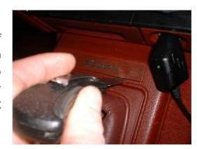
**2.** Remove the plastic trim piece surrounding power mirror adjustment knobs. We used a knife to remove these. Work slowly, this plastic is fragile. We suggest working your way around the trim pieces gradually instead of trying to remove the pieces in one shot. Place trim pieces to the side.
