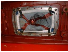
**6.** Emergency brake boot: Unsnap brake boot and remove. Snap is located at the bottom of the boot between passenger seat and console.
