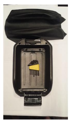
**15.** Once you remove the holding plate, you will see the vinyl assembly that is glued in place.... I chose to keep the old fake leather in place as RedlineGoods provides ample extra material to wrap around the factory fabric. There is NO NEED to remove it. You are going to wrap this with the new leather cover.
