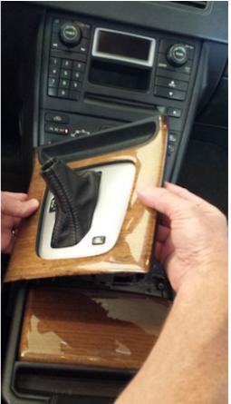
**12.** Tuck in the round boot frame inside the boot to attach (snap) in the base on the shift knob. Put a dab of grease on the end of the shift knob metal end before inserting back into the gear shift
