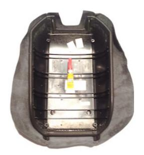
**17.** Insert the armrest tray back into and over the ends of the Leather.
