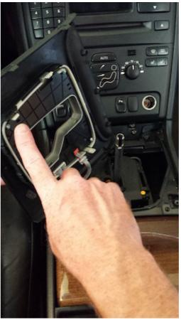
**4.** Remove the old boot from bottom of the gear shift plate by removing the frame.
