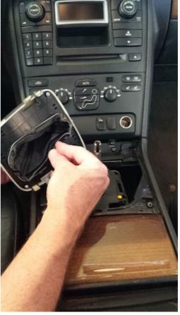
**6.** Alignt the cuts in the boot with the notches on the frame.
