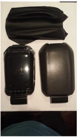
**16.** You need Super Glue to attach the new leatherto the base of the armrest. Lay out the Leather on the table Top Down, Place the armrest upside down in the center and work from the SIDES first. Small dab of Super Glue on one
