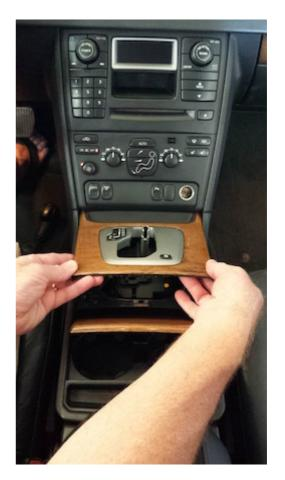
**3.** Turn the gear shift plate over and disconnect wire clips. Then look for the plastic taps that hold the silver gear plate to the wood frame. Separate the two.
