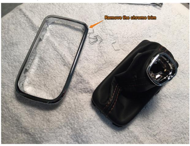
**7.** Very carefully separate the vinyl boot from the plastic bracket. The black plastic is thin, and you must take care not to snap it in two.
