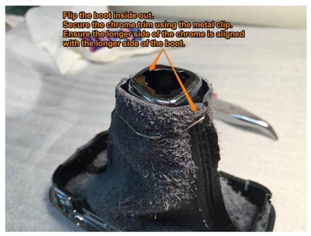
**18.** Flip the shift boot back to normal. Double check that everything is aligned, and that the chrome is positioned correctly.
