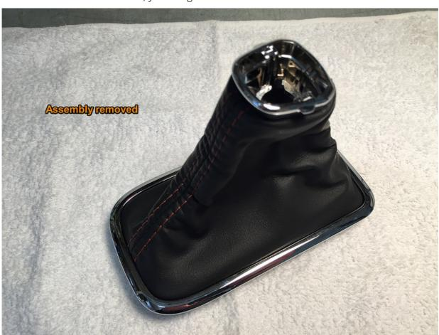
**5.** Straighten the legs on the staples which secure the vinyl boot in place.
