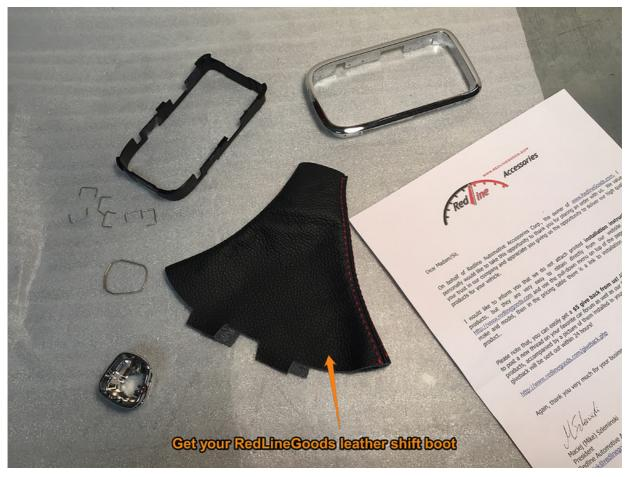
**11.** Test fit the black bracket into the shift boot. The boot has four tabs, the tabs will align with the little protrusions on the edge of the black bracket. You can also align the longer side of the boot with the more rounded side of the black bracket.
