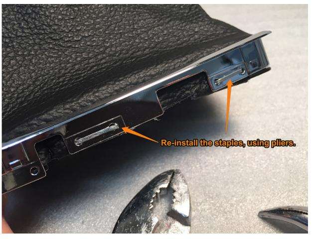
**17.** Flip the shift boot inside out. Line up the chrome trim such that the long side of the small chrome trim, aligns with the rounded side of the larger chrome surround. Take care not to install it upside down. The more narrow side should be clip with the edge of the leather trim. Secure the chrome with the wire clip, taking care to get the wire into the small channel in the chrome.
