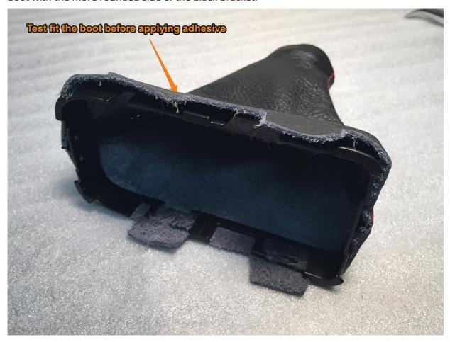
**12.** To properly secure the shift boot, use a fabric/plastic adhesive. I found the LocTite Flexible Fabric Adhesive to work great. You can purchase it at the hardware store. You will also need a 12 or 13 small binder clips.
