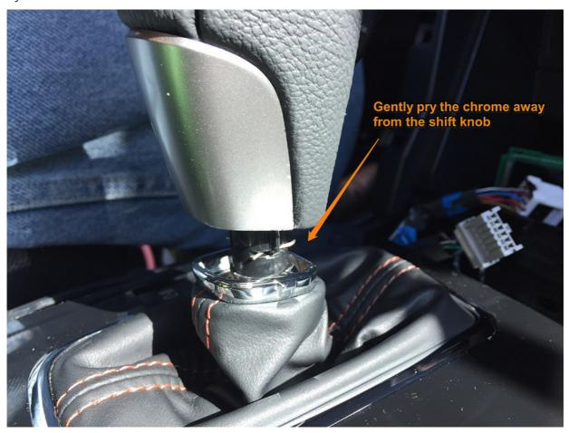
2. Remove the small metal clip which holds the shift knob in place. Do not loose this clip!
