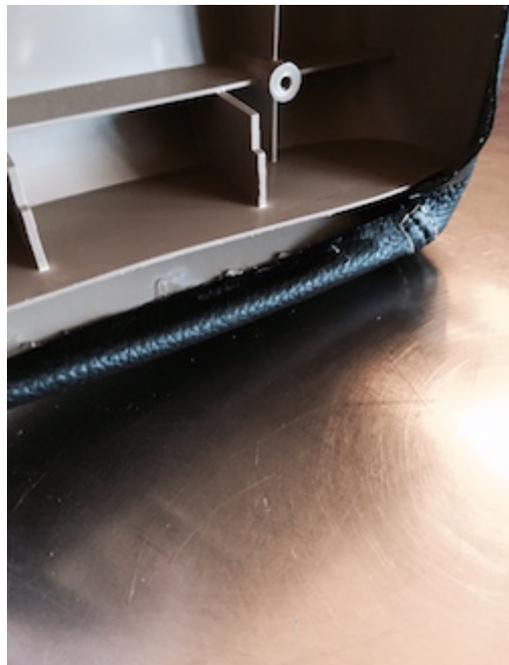
**13.** Once the glue is cured, reassemble the two halves of the lid. To finish off the area around the lock, glue it in. On version 2 you might need a grommet. Rowley Company #6 Black Rolled Edge Grommet is recommended. Works great but needs to be installed before attaching to console lid or you can't re-install the lock. With Grommet in place, still gives access to lock button to open console lid and room to get key into lock.
