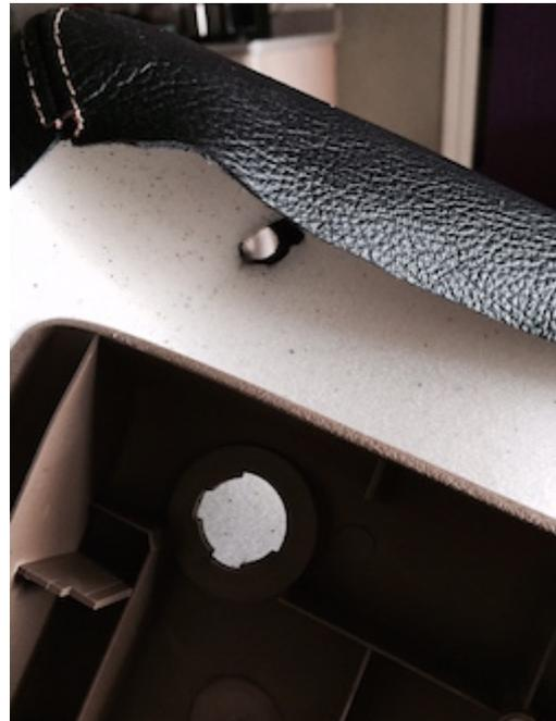
7. Apply glue (contact cement works great since it gives you a certain time for adjustments before it fully sets. Make sure to read the instructions for the glue you end up using so that you know what setting time it has.) to the top of the lid.
