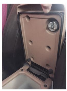
**2.** Remove screws at the hinge to take the lid off.
