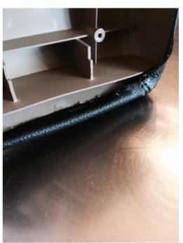
**13.** Once the glue is cured, reassemble the two halves of the lid. To finish off the area around the lock, glue it in. On version 2 you might need a grommet. Rowley Company #6 Black Rolled Edge Grommet is recommended. Works great but needs to be installed before attaching to console lid or you can't re-install the lock. With Grommet in place, still gives access to lock button to open console lid and room to get key into lock.
