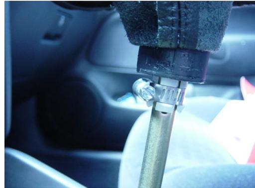
**6.** Remove the e-brake handle. Completely pull up the handle, pry back the tab on the bottom, and slide the handle off.
