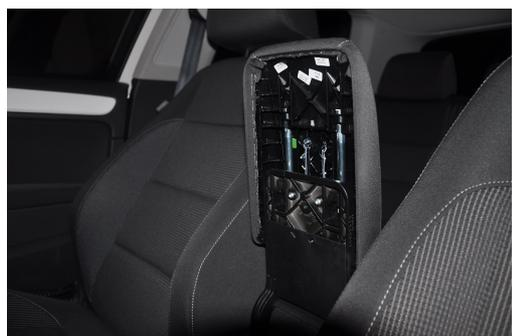
**4.** Unscrew the two screws and push/pull the arm rest cover down and up and it will slide off.
