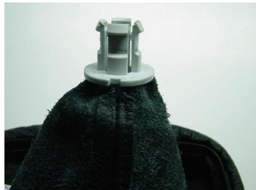
**4.** Slide the plastic retaining sleeve over the new cover and slide the shift knob back on to the shift lever. Push down until you feel it click into place.
