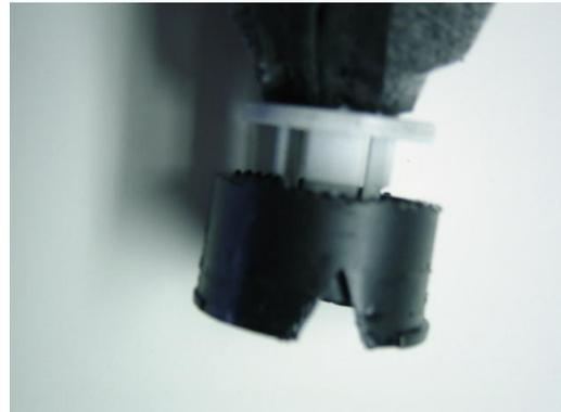
**3.** Remove the old boot and replace with the new leather boot cover.
