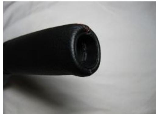
**8.** First, take out the inner plastic ring from the front of the handle by pushing it out from behind. I found a long flathead screwdriver worked well. Be sure to push from multiple points to avoid breaking the tabs off the ring.
