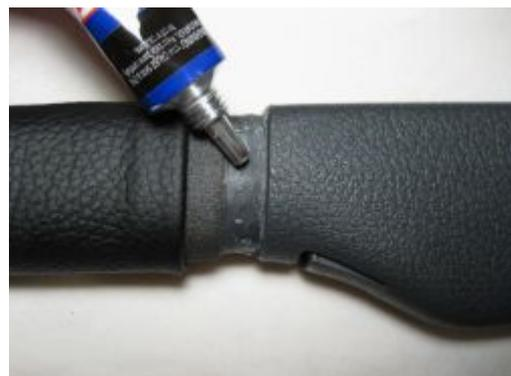
Reattach the front ring. After the glue has set, stretch the leather taut (just run your hand from back to front on the handle to remove any slack), and push the excess leather into the front hole of the handle. While still holding the leather, push the plastic ring back into its original position. Make sure you align the tabs correctly. This will take some force, as the new leather is thicker than the stock material.
