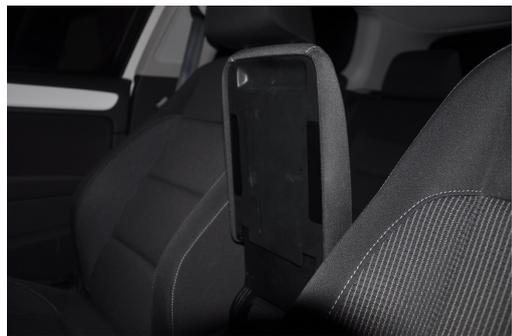
**2.** Grab the base of the plate and pull outwards. Top side swings out, but base and sides are simply clips.
