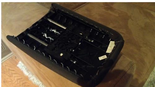
7. Remove the staples and peel back the OEM cloth cover and remove foam insert.
