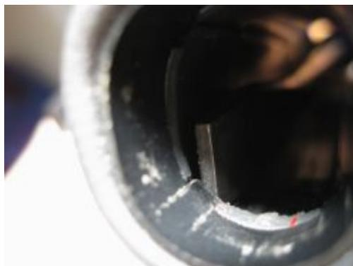
**10.** Scrape off the dry glue from the back of the handle to ensure the new cover holds firm.
