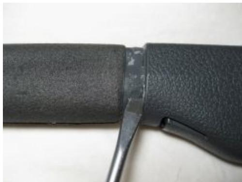
**11.** Glue the new cover to the handle. Slide the cover onto the handle almost to the very end. With the groove in the back of the handle still exposed, put glue in the groove and slide the cover the rest of the way on. Press the cover down onto the glue and hold according to the type of glue you are using. Make sure your glue is made for both leather and plastic.
