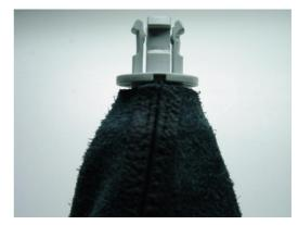
**5.** You will need to replace the metal ring, which held the knob in place. An easy replacement is a 1/4 - 5/8 in. hose clamp. Just place the clamp around the plastic prongs and tighten. Pull the cover over the shifter frame, re-install the frame back in place and you are done.
