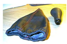
**3.** Working with the new leather shift boot, flip the boot inside out and slide the 1" top opening over the bottom recess of the shift knob. Use a thin plastic zip tie or equivalent and wrap around the recessed part as pictured below. Once you are done, invert the shift boot back to normal and pull down on the leather boot to position it the way you want.
