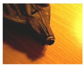
**4.** Screw the shift knob back onto the gear shaft clockwise until you have it at the normal position. Lastly, stretch the elastic bottom of shift boot to fit over the console recess and you are done.
