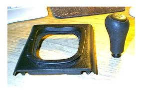
**2.** Unscrew the OEM shift knob by turning counter-clockwise until you are able to pull off the knob and boot together from the gear shaft. Remove the old shift boot by pulling it off the shift knob.
